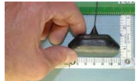
Figure 2. Location-only Argos tag for attachment to cetacean dorsal fins.
