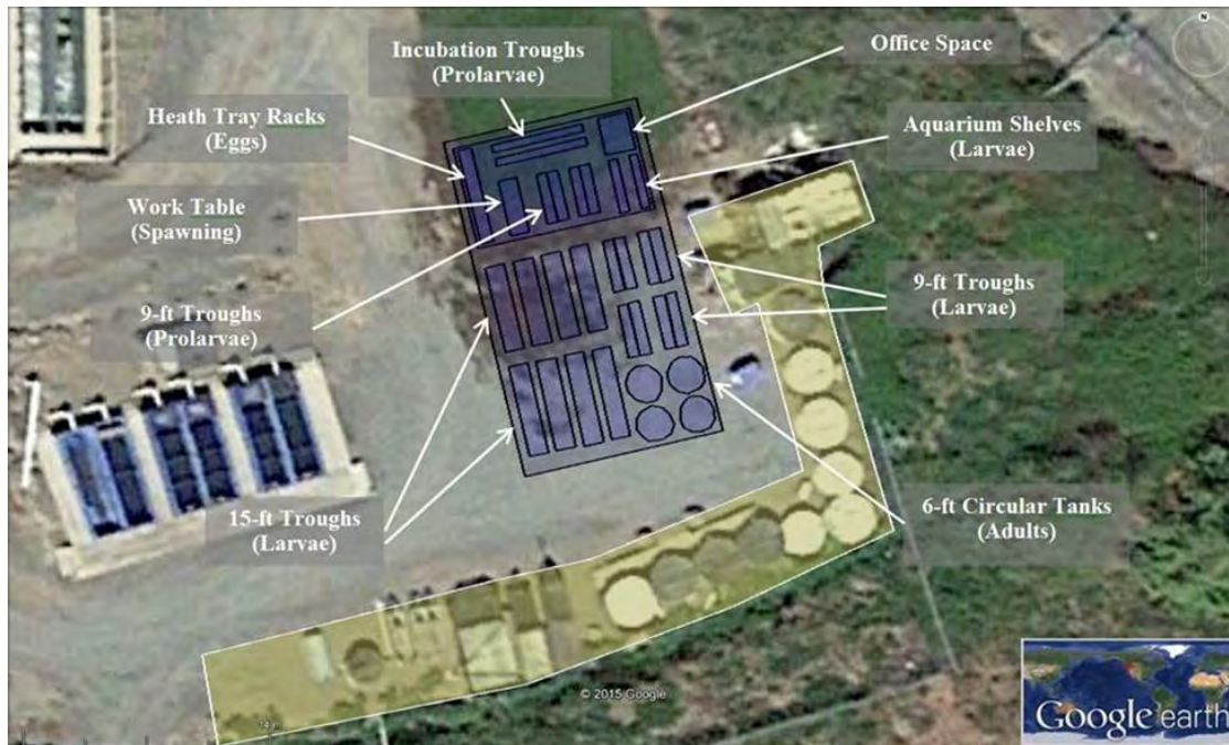
Figure 5-7. Aerial overview of the new pole building and tanks proposed at the East Lamprey Facility at Prosser Fish Facility.
