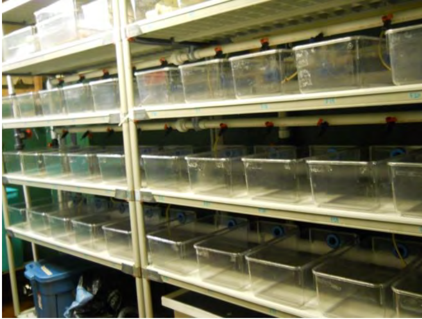
Figure 5-13. De-watered lamprey rack system at MUK with 30 replicate polycarbonate tanks.
